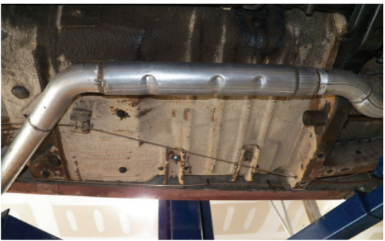
A mock-up on another B-body showed that 'Sticks are slender enough to be installed as resonators, next to the fuel tank.
