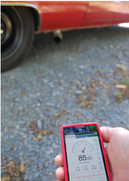
At 1,500 RPM, with the meter 4 feet from an outlet, we measured a loud 85 decibels. At WOT it was way louder. This was our baseline.
