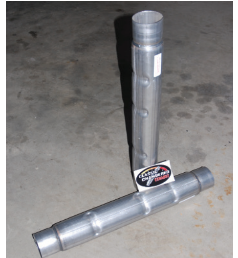
We hoped a pair of 3" Powersticks (they come in a wide variety of lengths and diameters), straight-through chambered mufflers from classicchambered.com, would reduce the noise to a tolerable level.
