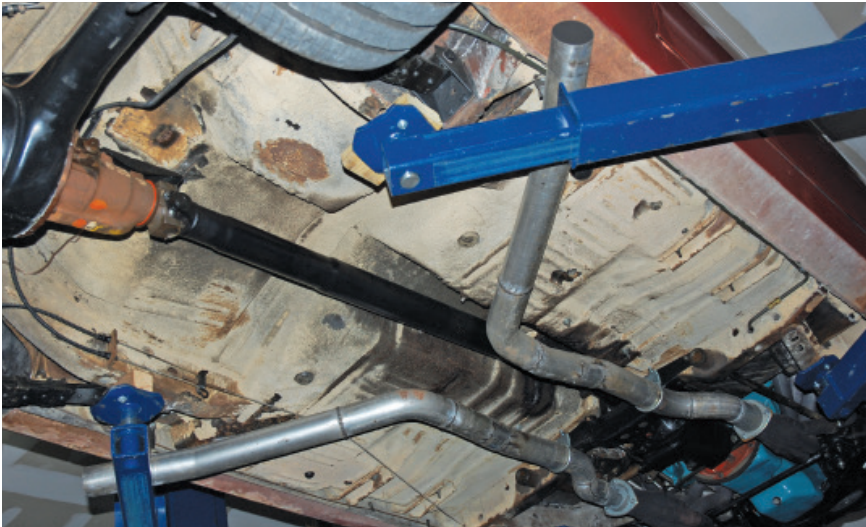
Sals' exhaust system, if you can call it that, was a hand made NASCAR-style setup. Wide open. And loud.
