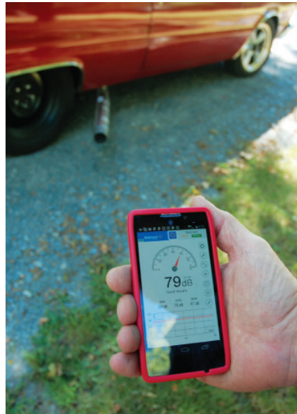
With a P'Stick stuck on, we lost 6dB. Noticeable in anyone's book.
